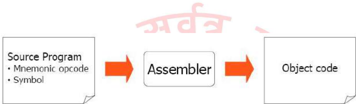
Figure 1. Executable program generation from an assembly source code
