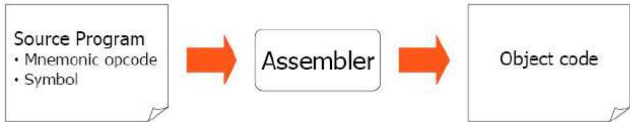
Figure 1. Executable program generation from an assembly source code
